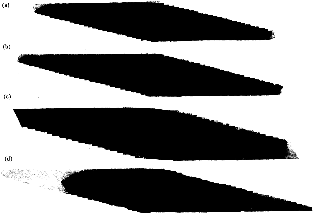
Fig. 3. Photographs of layer surfaces deformed in simple shear taken at \gamma = 3.8 , seen in the XZ plane: (a) model with viscosity ratio 30:1 and an initial planar layer, (b) model with viscosity ratio 30:1 and an initial domed perturbation, (c) model with viscosity ratio 30:1 and an initial cylindrical perturbation, (d) model with viscosity ratio of ca. 600:1 and an initial planar layer. The initial spacing between the grid lines in all models was 5 mm in the undeformed state.
